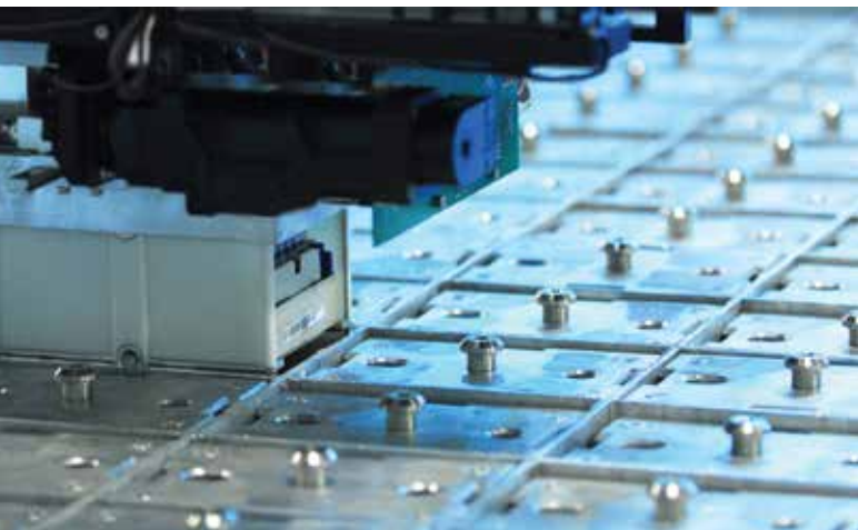
▲ The internal robotics of the Hamilton BiOS system manage stacks of tube racks as part of the automated storage and retrieval process. (Image courtesy of Hamilton Storage Technologies.)
