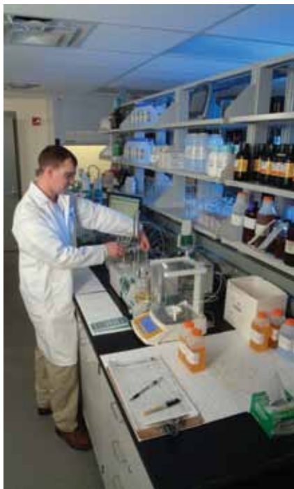
▲ In-process testing and validation with automatic potentiometric titration, Karl Fisher titration, and manual titration.
