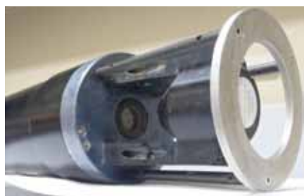
▲ A laser particle analyzer to determine the concentration and particle size distribution suspended in water (Source: Matthew Sullivan)
