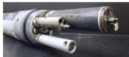
▲ An optical dissolved oxygen sensor on a multi-parameter water quality meter that is configured for logging dissolved oxygen, pH, conductivity, and temperature. (Source: Matthew Sullivan)
