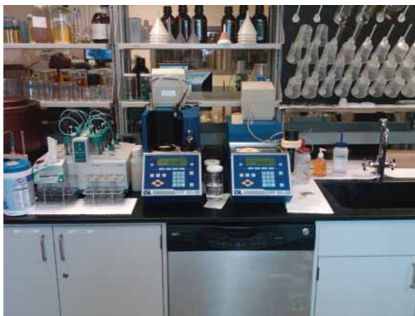
▼ The HERO BX laboratory houses many automatic physical property testing instruments such as cloud point, flash point, viscosity, and cold filter plugging point.
