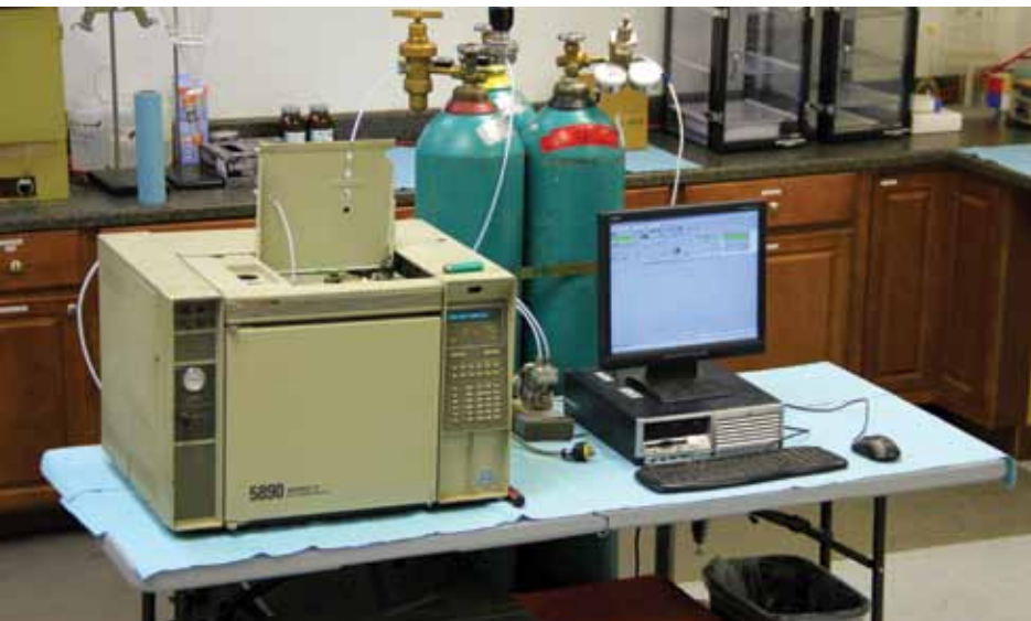
▲ 5890 Gas Chromatograph with FID used for EPA Method 18
