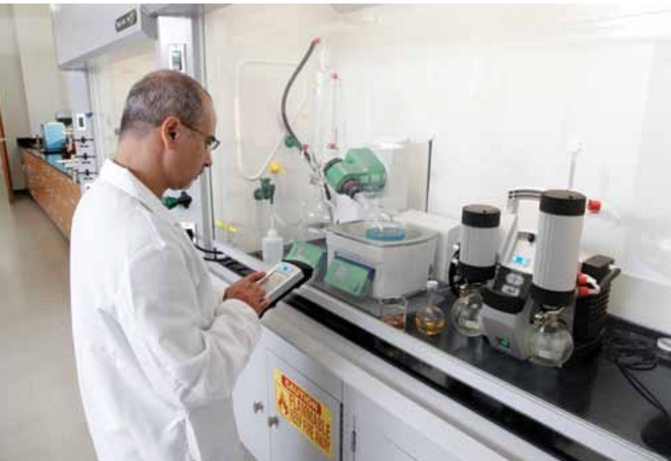
▲ Using Bluetooth technology, KNF's SC920 vacuum pump can be used inside a hood with the sash closed. (Image courtesy of KNF Neuberger)
