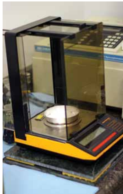
▲ Analytical balance used for gravimetric analysis in the Airtech lab.
