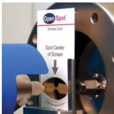
▲ Mass Spectrometry Source / DART®-OS / IonSense / www.ionsense.com
