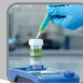
Step 5 If required the sample can be extracted for analysis with a syringe through the pierceable membrane of the tube lid.
