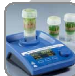
Step 3 The mint leaves are homo- genized by the rotor-stator unit in the DT Tube.
