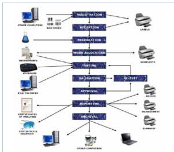
◀ Figure 3. Key functional steps in configuring a LIMS.
