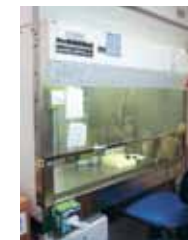
▲ The Baker Company's SterilGARD® III Class II Type A2 biological safety cabinet from 1998.
