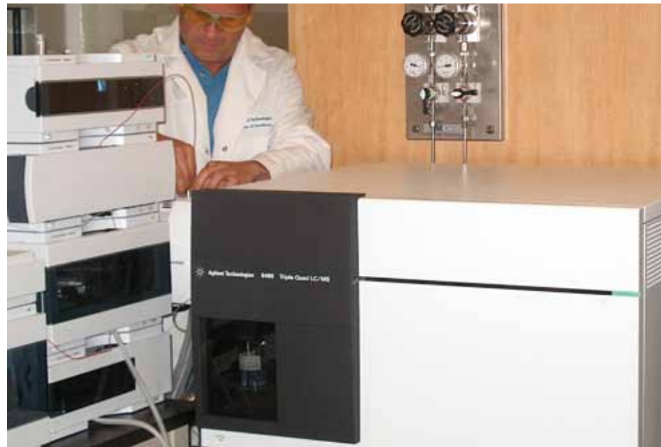
▲ The Agilent 1290 Series UHPLC used in conjunction with a 6490 triple quadrupole mass spec, a workhorse category instrument used throughout the food testing industry.
