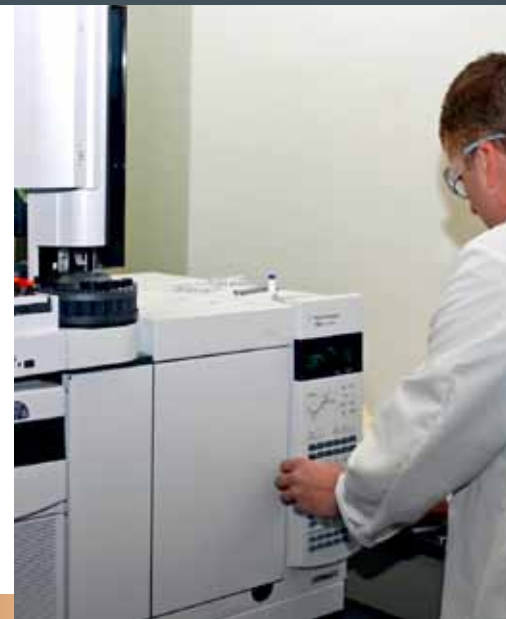
▲ The Agilent 5975C GC/MS, a popular platform for detecting and identifying food contaminants such as pesticides on fruits and vegetables.
