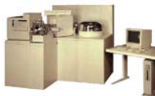
Finnigan's MAT 90, the first mass spectrometer to be completely controlled by computers.
