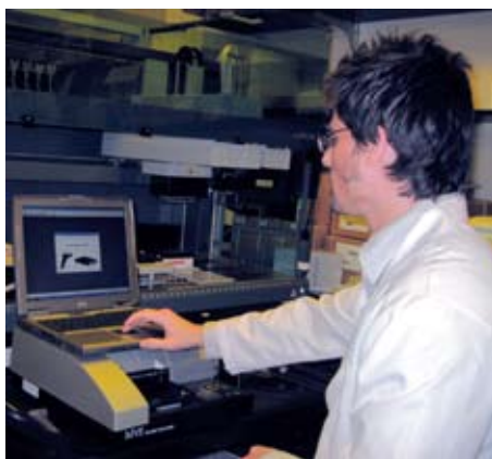
▲ Xenotech research scientist of R&D / Method Validation of Laboratory Automation, Robert T. Grbac, using the Artel MVS® to measure the accuracy and precision of his automated liquid handler.
