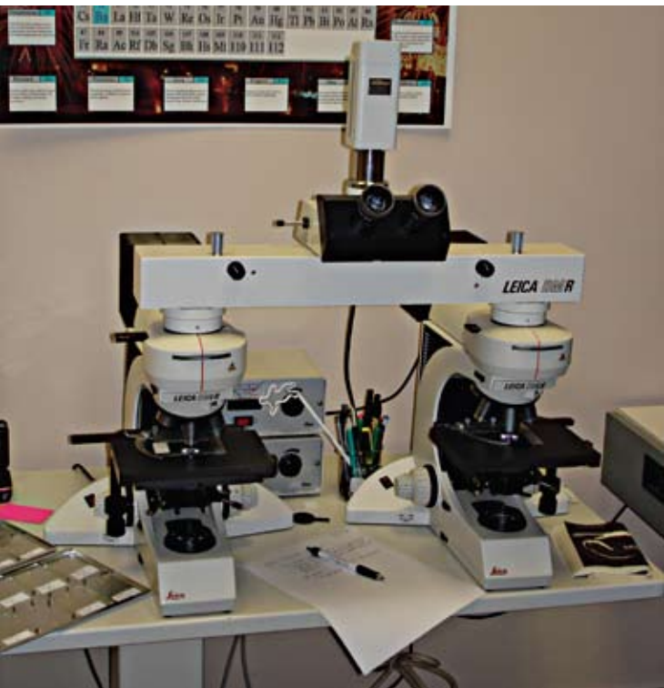
▲ The Tarrant County Medical Examiner's forensic lab's comparison microscope used in trace analysis. Photo credit: Larry Reynolds
