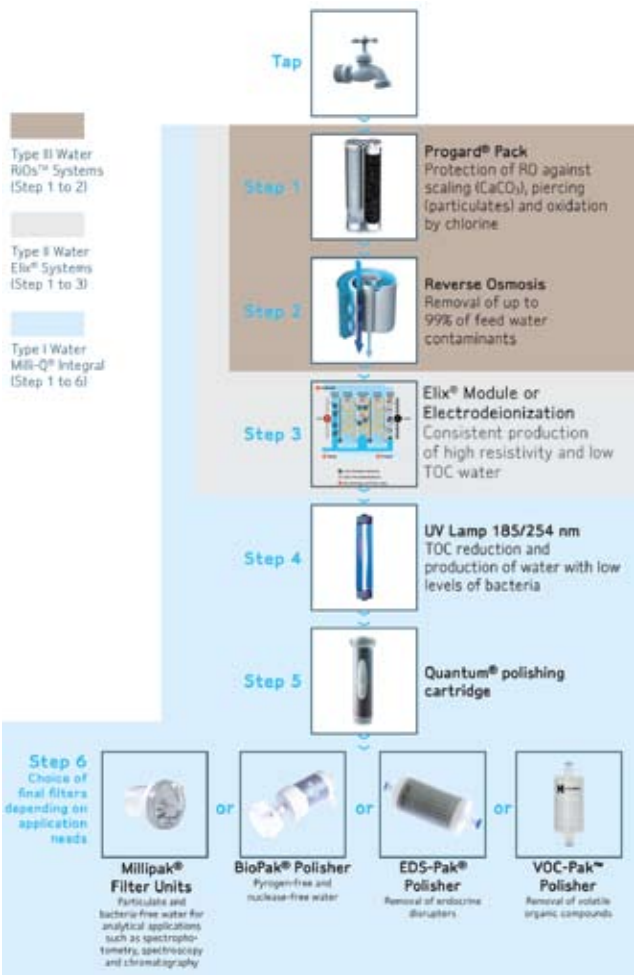
▲ Figure 5. Multi-step purification process required to achieve different water quality levels.
