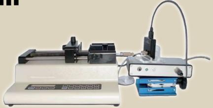
▲ RheoSense's new micro-liter viscometer using lab-on-a-chip technology
