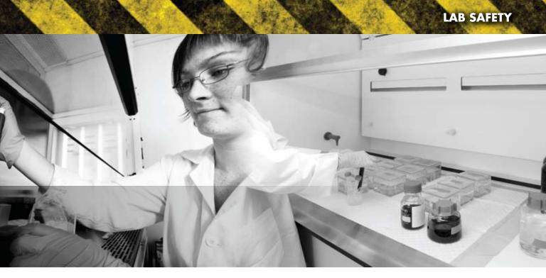
However, as the sash is closed, velocities can increase to the point where they disturb instrumentation and delicate apparatuses, cool hot plates and slow reactions, or create turbulence that can force contaminants into the room.
