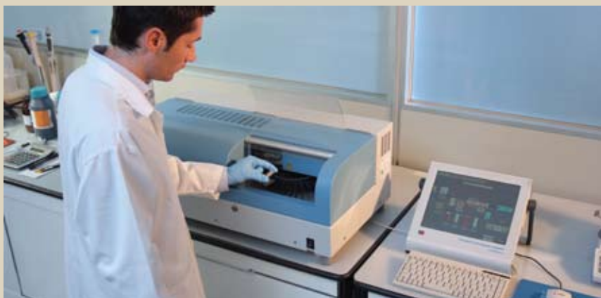
▲ Milestone's DMA-80 Direct Mercury Analyzer allows for prep-free, matrix-independent analysis in as little as five minutes.
