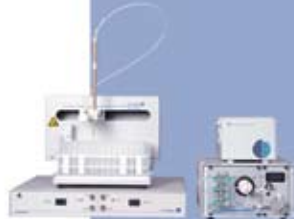
CNSolution™ Cyanide Analyzer Measures total cyanide without distillation in minutes by ASTM Method D7511-09
