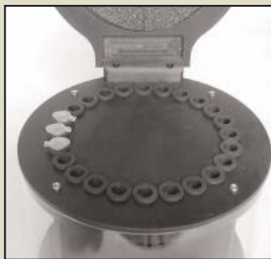
Figure 2. The Bullet Blender™ can process up to 24 samples in closed tubes at once.
