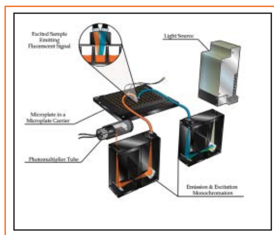
Figure 2. Monochromator-based Detection System in a Multi-mode Microplate Reader
