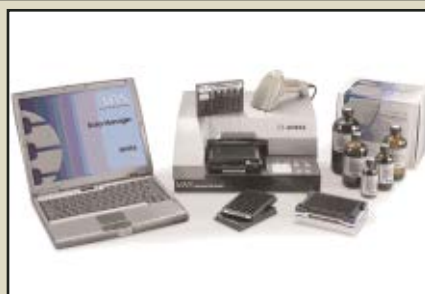
Figure 2: ARTEL's MVS (Multichannel Verification System) verifies the performance of automated liquid delivery devices.
