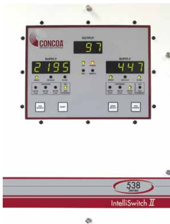
▲ CONCOA's IntelliSwitch II controls and monitors cryogenic supply systems.
