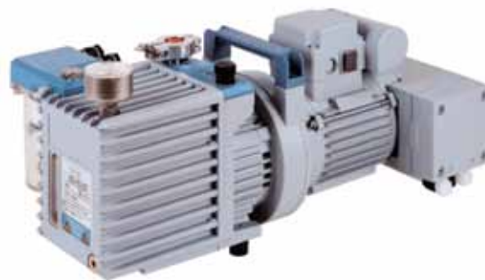
▲ VACUUBRAND RC6 Chemistry-HYBRID pump. Hybrid vacuum pumps, combining rotary vane and diaphragm technology, provide deep vacuum levels with greatly reduced service.
