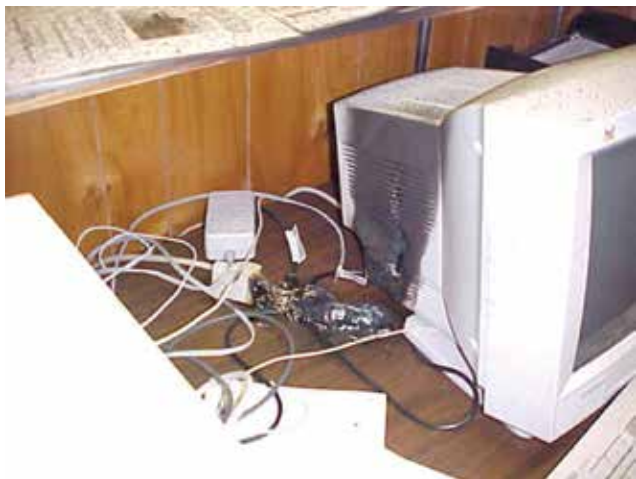
▲ This fire started with the MOV-based surge suppressor. Fires such as this prompted a 15 million-unit recall in the fall of 2013.
