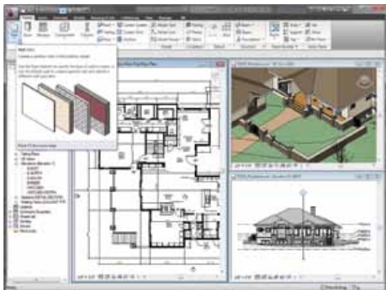
▲ Drawing a wall in BIM. Image Source: Cunba, 2012.
