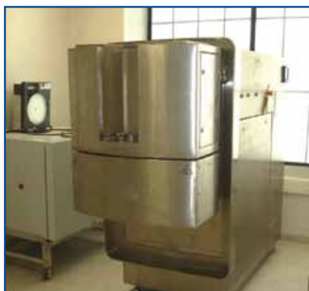
25 Liter GEA Collette NV High Shear Mixer, Type UltimaGral 25, S/S
