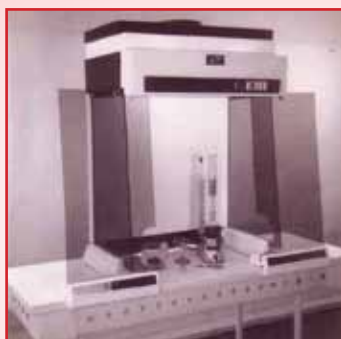
◀ The first ductless fume hood, invented by Erlab in 1968, had filtration capabilities that were limited to just a few chemical contaminants of the same family.
