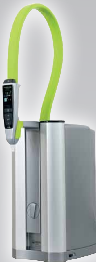
▲ The PURELAB flex delivers 18.2 MΩ-cm water quality.
