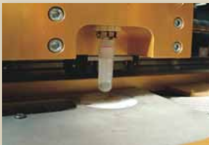
▲Robot gripper holding the vial.
