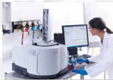
▲The Thermo Scientific iPRO 5000 Series Total Nitrogen/Total Sulfur (TN/TS) analyzer.
