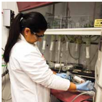
▲ Technician extracting fat for food using the traditional soxlet method.
