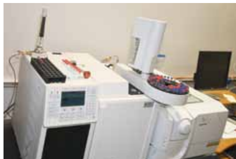
◀ Varian Triple Quad 320 Gas Chromatograph Mass Spectrometer/ Mass Spectrometer, the NFL chemistry department's work horse.
