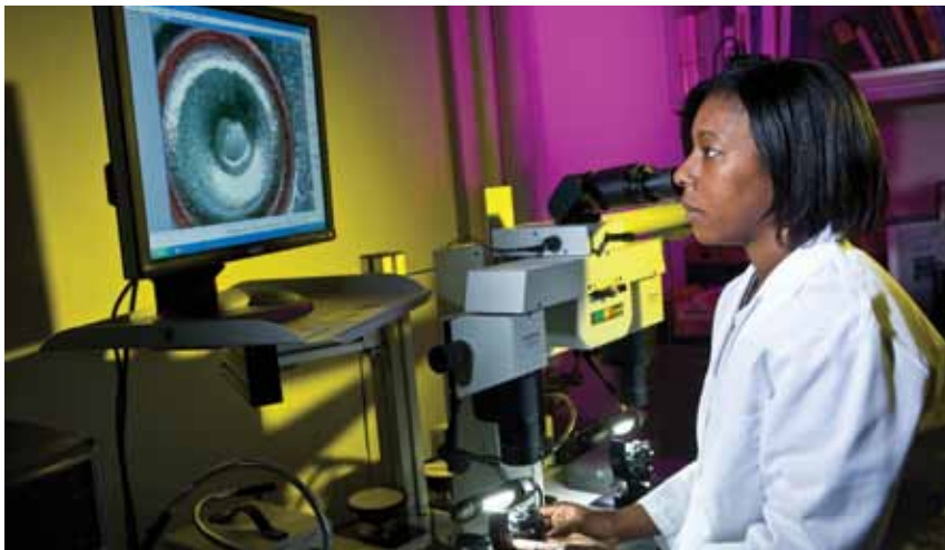
▲ Firearm and Toolmark Examiner Shirley Marc examines a firing pin impression using a comparison microscope.
