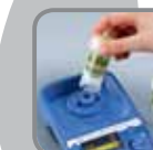
Step 4 Test result: The mint leaves are dispersed homogeneously. The tube is removed from the drive system.
