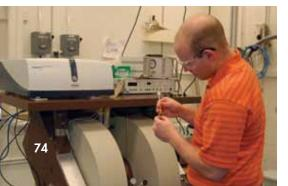
Combustion elemental analysis involves burning a solid sample to produce carbon dioxide, hydrogen and nitrogen. Measuring the amounts of these gases produced enables researchers to determine the absolute percentages of carbon, hydrogen and nitrogen in the sample.
