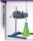
▼Eberbach's Model 7225 Con-Torque Stirrer is suitable for continuous duty stirring of highly viscous materials. A 1/9 hp motor and gear drive produces 196 oz-in of continuous torque which drives the hollow spindle through a speed range of 0 to 700 rpm.
