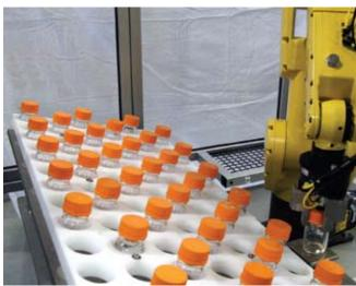
After the bottle is agitated, the robot places it on an integrated scale that records data to a PC.
