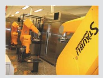
Fully automated, ultra-high-throughput robotic screening systems from Kalypsys Inc., currently in use at the laboratories of the Chemical Genomics Center at NIH. (Source: Marc Ferrer, Ph.D.)
