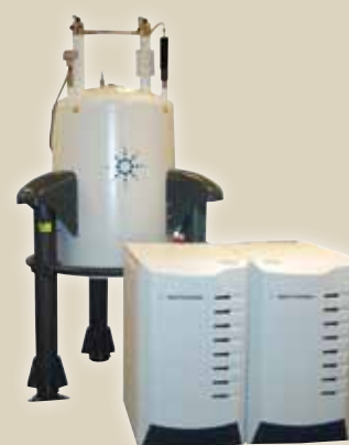
▲ Typical solid-state NMR equipment. Shown is the 600 MHz NMR system with Direct Drive 2 console, an Agilent solid-state NMR machine.
