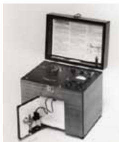
A Beckman Model G Acidimeter from 1936, later renamed the Model G pH meter. Courtesy of Beckman Coulter, Inc.
