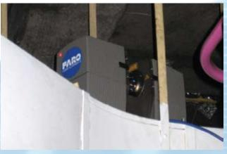
◆ Scanning equipment can document hard-to-reach spaces such as behind ductwork or above the ceiling.
