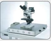
Vibration-Free Platform provides a portable isolation system wherever you need it.
