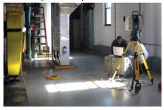
▲ Laser scanners connect directly to a laptop, allowing users to see the results of the scans almost instantly.
