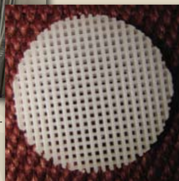
▲ PCL scaffold with pore size ~ 500 microns.
