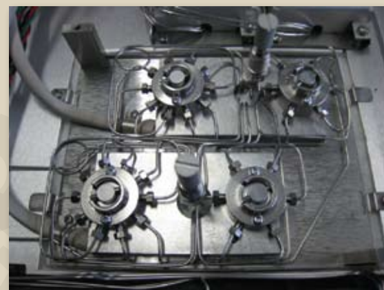
◀ Complex valve configuration typical of customization supplied on some analyzers.
