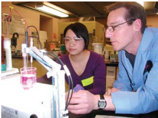
▲ Joe Curran, research chemist, at Ashland's Dublin facility, trains Wanxing Nancy Ni, chemist, Ashland Shanghai Technical Center, in performing acid value titrations.
