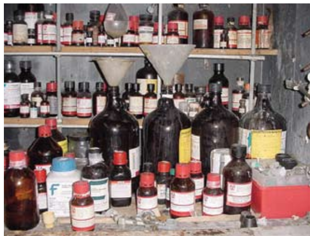
▲ A host of problems, from inappropriately stored waste to blocked hood baffles, unlabeled and mislabeled containers to residual spills. Photo courtesy of Mark Yanchisin
