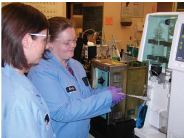
▲ Holly Sennhenn, senior research chemist, watches as Emily Stawicki, technician, prepares a sample for distillation to determine nitrogen content using the Kjeldahl method of nitrogen analysis.
