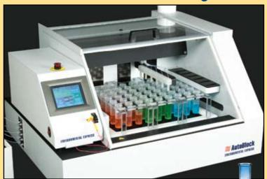
he AutoBlock™ from Environmental Express accurately adds concentrated acids and heats and cools samples in a HEPA-filtered environment. Use one of the EPA Methods stored in permanent memory or easily program and store your own methods.
